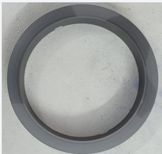
Figure 2: Narrow Contact Band on Sealing Surface (Mating Ring)
