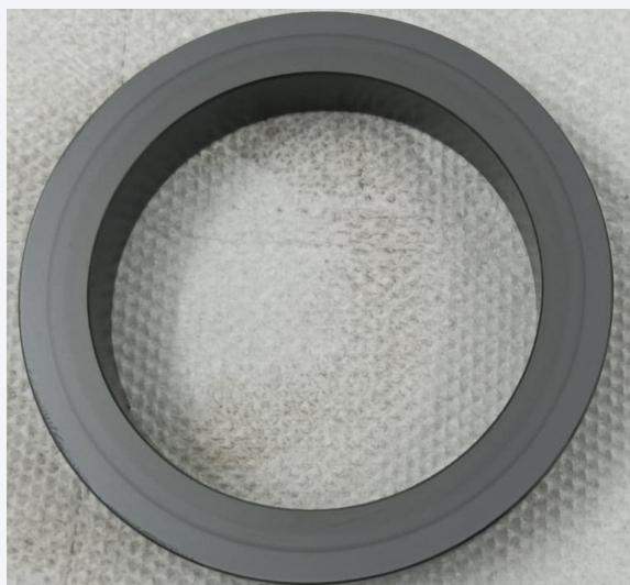
Image 2: Narrow Contact Band on Sealing Surface (Mating Ring)
